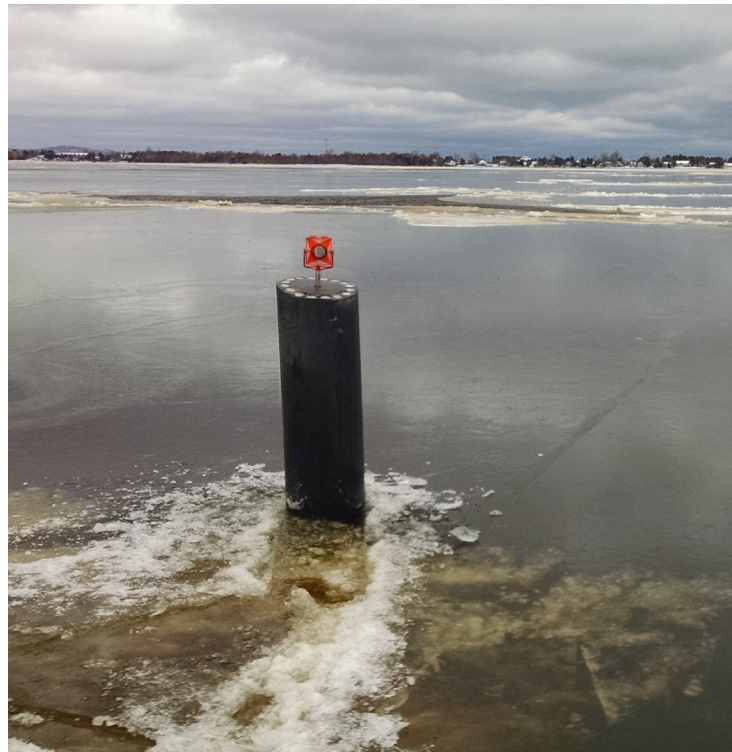
Figure 2: Test Pile Resisting Ice Movement in Dec. 2015
