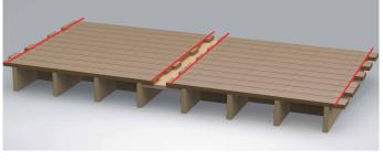
Once TanDeck has been installed on both sides of the feature board cavity, snap two lines where the feature board will be positioned. Consult gap chart to determine proper width of feature board cavity. Snap lines to mark clean edges at the over hangs.
