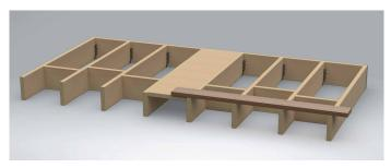
Mark where the feature board will be positioned with two chalk lines. Install TanDeck long protruding into the feature board cavity.
