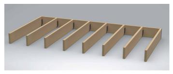
Set joists at 16" on center or less when installing 5/4x6 or 24" on centers, or less for 2x6.
