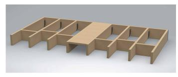
2 Joist should be supported with joist bracing every six foot. Install solid bridging between the joists below where the feature board will be installed, per your designed layout.
