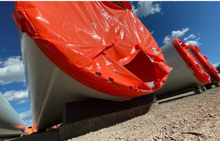
Tangent cribbing with custom cut saddles supporting 240,000 lb GE wind turbine towers
